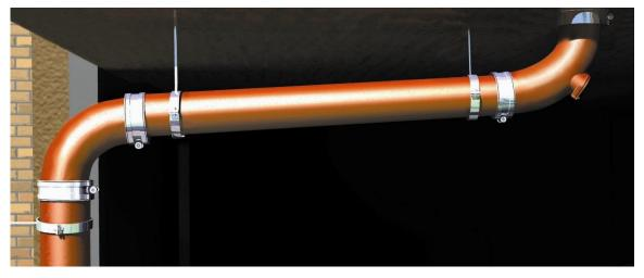
The normal recommendation for gradient on 100mm pipes is 1:40 minimum fall and 150mm pipes 1:60 minimum fall. The pipe should also be supported at every change of direction or branch connection and in some cases, it may be necessary to provide a lateral brace at 12m intervals. The max length of threaded rod for a single drop bracket should be 750mm; for longer drops it is recommended two drop rods are utilized with a split band clip.
