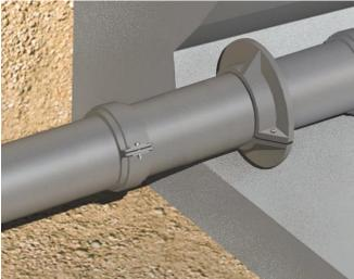
In basement areas where pipes pass through external walls it may be necessary to install a puddle flange. For locations which are below the water table or in areas liable to flooding, puddle flanges will reduce the risk of water entering the building.
