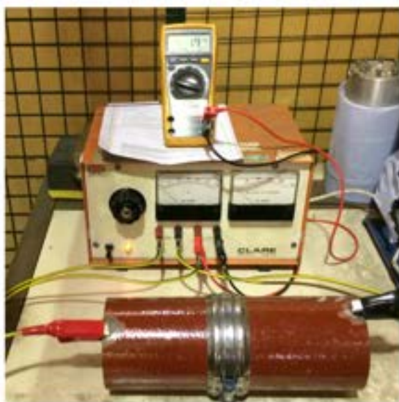
Electrical Continuity Testing
